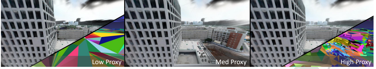
Figure 9: Impact of the spatial resolution of the proxy mesh (low to high from left to right) on the ArtSci scene. The medium proxy mesh (not shown to provide a full view of the scene) is inbetween both extremes in terms of the numbers of faces.
