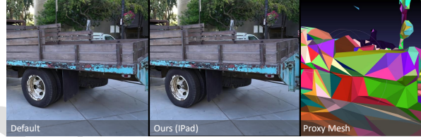
Figure 1: 3D Gaussian Splatting of the well known truck scene [1], render using the original implementation vs. ours running on mobile together with our generated proxy mesh to determine visibility.
